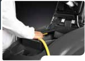
The periodic cleaning of the suction hose ensures an efficient drying over time
